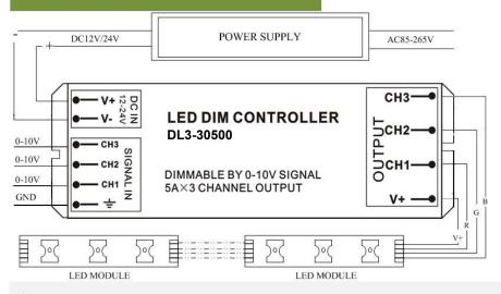
△ Note: This unit can be connected with various single-color modules and common anode connected full-color modules.
