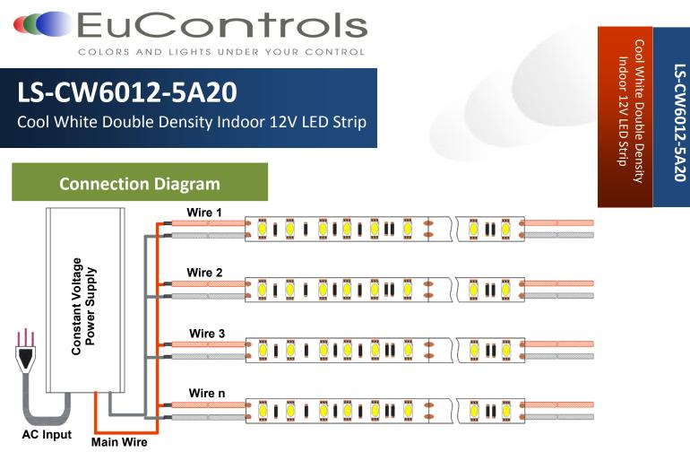
**Note:** For consistent brightness and even appearance, we recommend you to connect the LED strips to a power supply or repeater every 20-30 ft. to minimize voltage drop.
