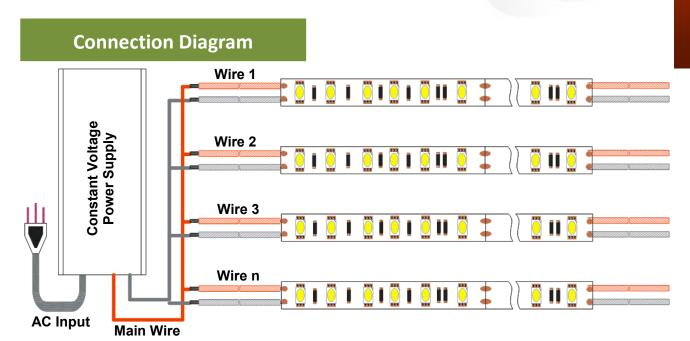
Note: For consistent brightness and even appearance, we recommend you to connect the LED strips to a power supply or repeater every 20-30 ft. to minimize voltage drop.
