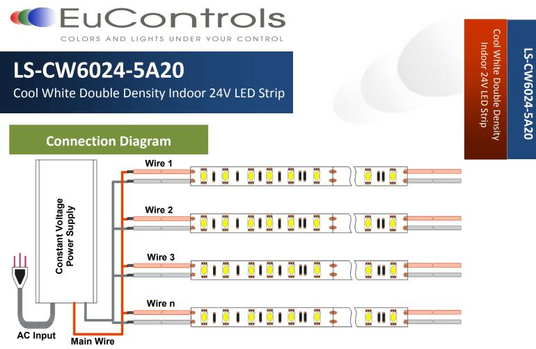
**Note:** For consistent brightness and even appearance, we recommend you to connect the LED strips to a power supply or repeater every 20-30 ft. to minimize voltage drop.
