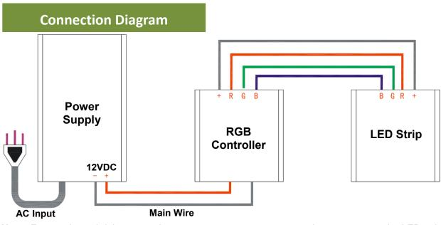
**Note:** For consistent brightness and even appearance, we recommend you to connect the LED strips to a power supply or repeater every 20-30 ft. to minimize voltage drop.
