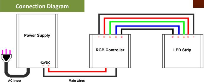
**Note:** For consistent brightness and even appearance, we recommend you to connect the LED strips to a power supply or repeater every 20-30 ft. to minimize voltage drop.
