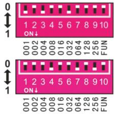
Example 1, DMX512 initial address code 37 means that the value of switch 1, 3 and 6 is "1", and the value of the rest of switches is "0", so the total value of the switches is 1+4+32=37.
