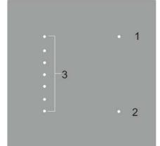
**[Power ON]**: Touch-sensitive **Zone 1** is used for power on. The dimmer memory will remember the brightness level.
